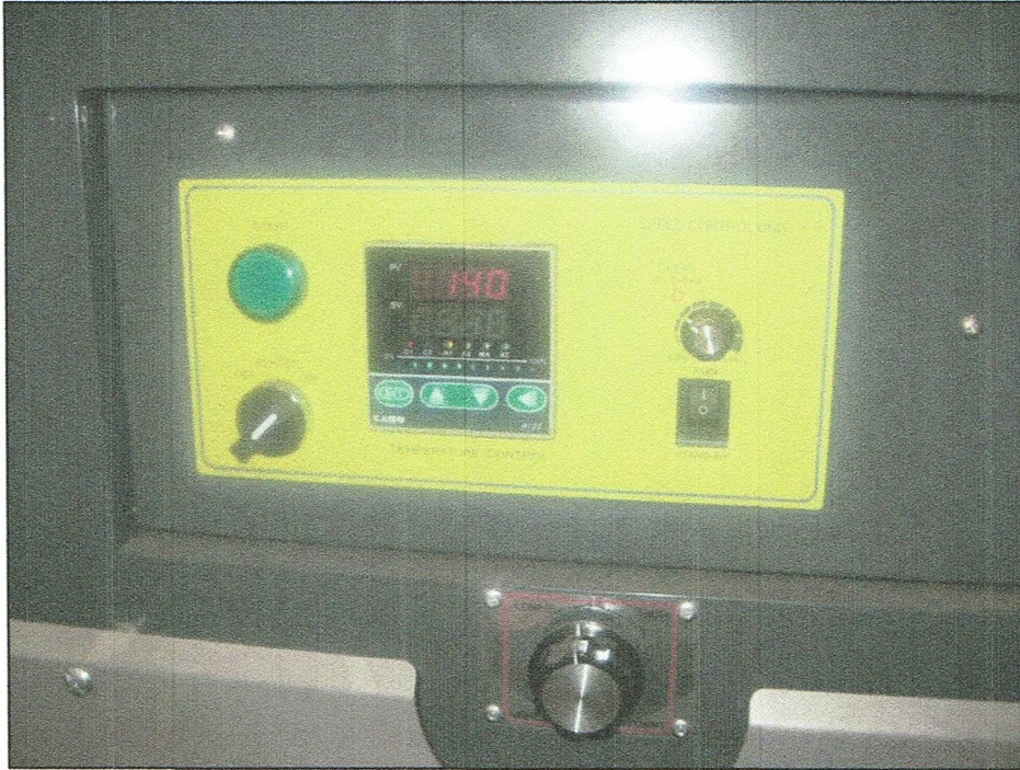
Photo 12: XEKL 455 MT: Heating tunnel controls with ON/OFF and conveyor speed
