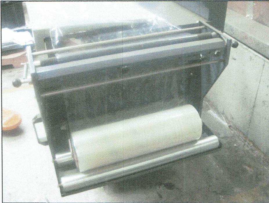
Photo 2: XEKL 455 MT: Shrink wrap unloader side
